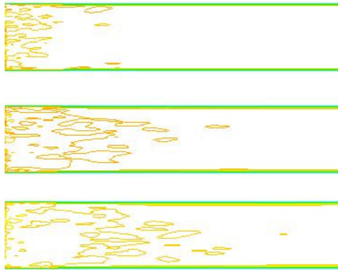
Figure 3.8: Propagation of turbulence from the inlet to the interior region of the pipe.
